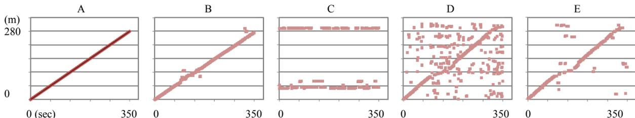
Figure 4. System estimations for user position while traversing a set path. In other words, plots show position (vertical) during a certain time (horizontal). Plots are A) ground truth (actual position), B) constant speed, C) speed is constant but there is a shift in magnetic field, D) the same as C, but with our shift compensation algorithm, E) the same as C, but with both shift compensation and outlier replacement applied.
