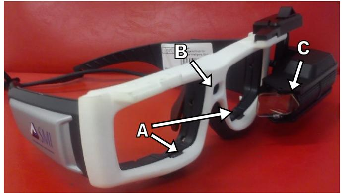
Figure 3. System setup showing A) inward facing cameras, B) outward facing camera, and C) HMD.
