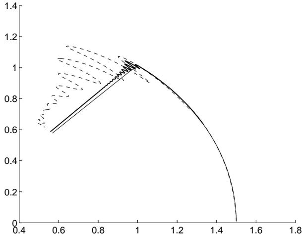
Fig. 8. End-effector trajectories. Thin solid line: Controller using SDS scheme and perfect inverse dynamics. Dashed and bold (wavy) lines: Controller using SDS scheme external space parameters. SDS parameters for dashed and thin solid lines:  $\alpha = 100$ ,  $\Lambda = 30$ , for bold line:  $\alpha = 600$ ,  $\Lambda = 100$ .
