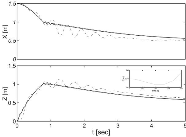
Fig. 7. Coordinates of end-effector versus time. Thin solid line: Controller using SDS scheme and perfect inverse dynamics. Dashed and bold (wavy) lines: Controller using SDS scheme external space parameters. SDS parameters for dashed and thin solid lines:  $\alpha = 100$ ,  $\Lambda = 30$ , for bold line:  $\alpha = 600$ ,  $\Lambda = 200$ . The inset depicts the initial perturbation of the controller caused by the weight of the arm observable for the dashed line.
