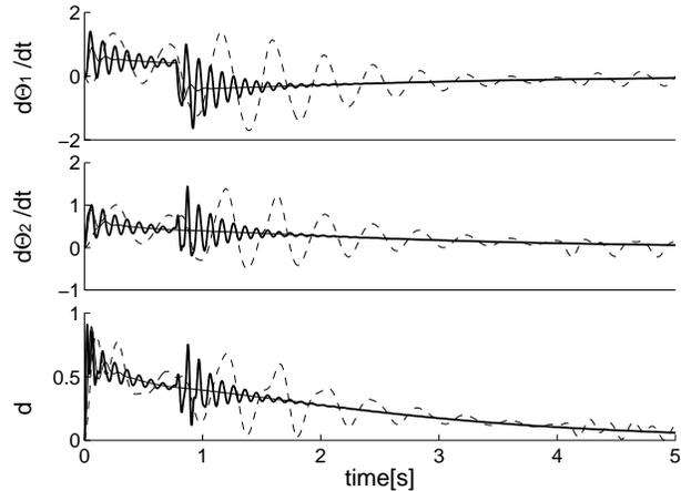
Fig. 6. Joint angular velocities versus time. Thin solid line: Controller using SDS scheme and perfect inverse dynamics. Dashed and bold (wavy) lines: Controller using SDS scheme external space parameters. SDS parameters for dashed and thin solid lines:  $\alpha = 100$ ,  $\Lambda = 30$ , for bold line:  $\alpha = 600$ ,  $\Lambda = 200$ .
