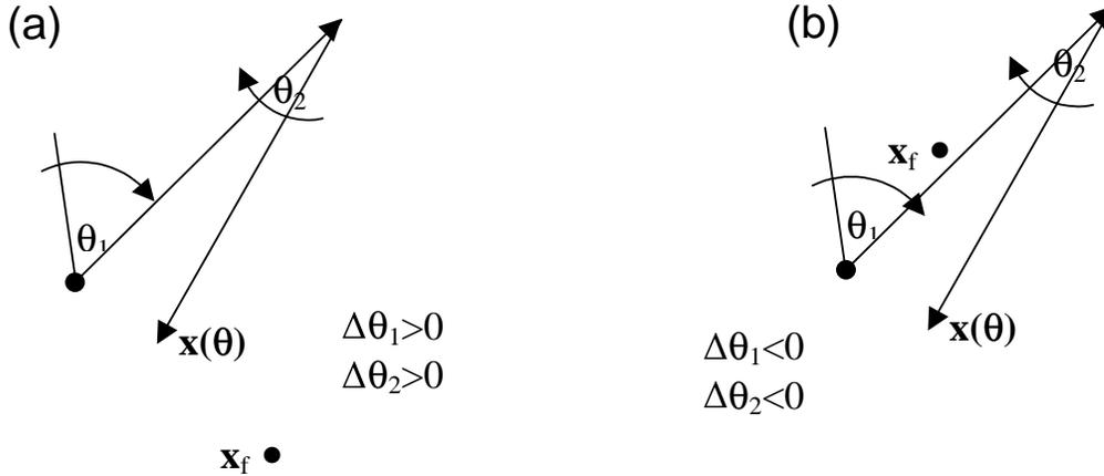
Fig. 4. Control signal in different configurations. (a) The end-effector  $\mathbf{x}(\Theta)$  can be moved closer to the desired point  $\mathbf{x}_f$  by increasing both angles. The arm will not be trapped. (b) The end-effector  $\mathbf{x}(\Theta)$  can be moved closer to the desired point  $\mathbf{x}_f$  by decreasing both angles. The arm will be trapped. However, if angle  $\Theta_1$  is kept constant at the early stage of motion then the same method will avoid the trap.
