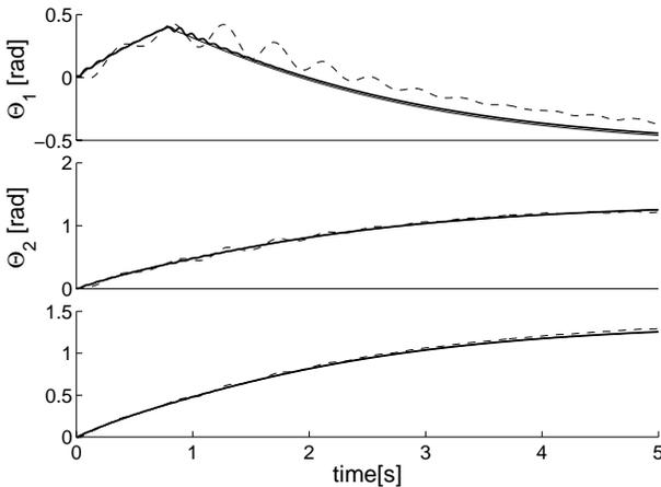
Fig. 5. Joint angles versus time. Thin solid line: Controller using SDS scheme and perfect inverse dynamics. Dashed and bold (wavy) lines: Controller using SDS scheme external space parameters. SDS parameters for dashed and for thin solid lines:  $\alpha = 100$ ,  $\Lambda = 30$ , for bold line:  $\alpha = 600$ ,  $\Lambda = 200$ .
